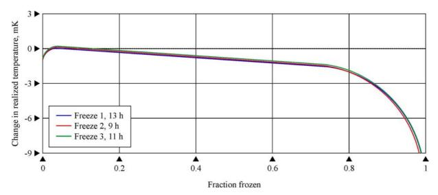
Graph 2. Freezing curves for the Isotech Al fixed point cell (Isotech model ITL-M-17672-O, Serial No. Al 188
